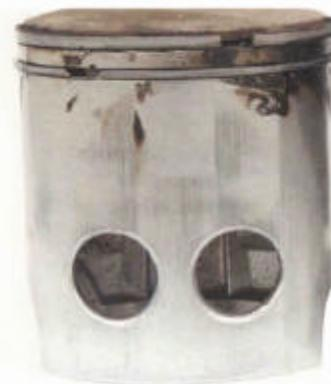
Piston from engine run on ValvTect Marine Gasoline
