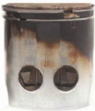
Piston from engine run on typical automotive gasoline
