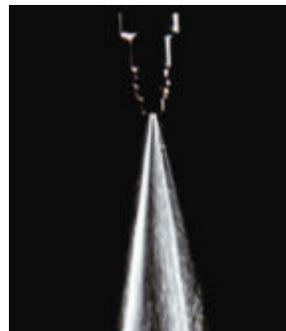
Partially Clogged Injector with automotive gasoline
