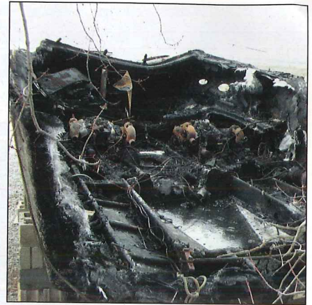
This boat caught fire when a grinder sparked a gas vapor explosion at a New Jersey boatyard.
